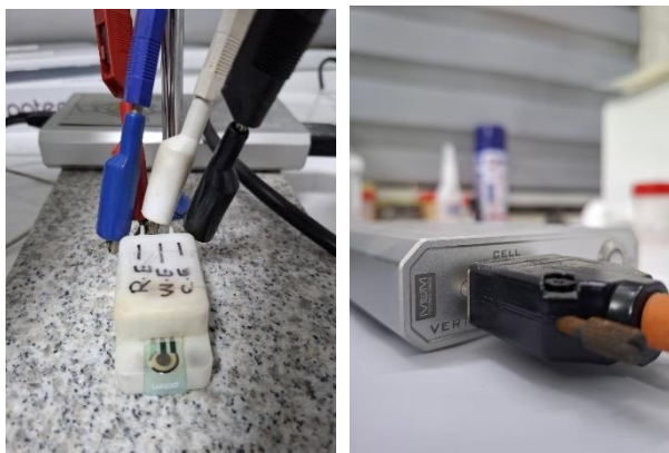
Fig 2: Steps of setting up and connecting electrochemical cell
