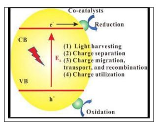
**Figure 1.** This figure shows the four fundamental stages of photocatalysis [11].
